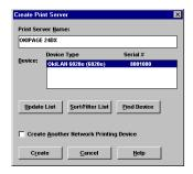
Note: If the Device list box is still empty, select Find Device. This will allow you to locate the specific device you are trying to define. You will be prompted for the Ethernet address and network number of the device. A mismatch in the OKI device frame format may cause the device not to show up in the Device list box.
